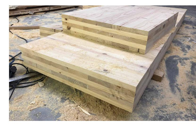
We manufacture our cross Laminated Timber is made in accordance with the requirments of SANS 8892. After the panel is machined the dimensions shall be within the following tolerances:
